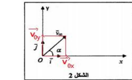
$$\vec{v}_G \left| \begin{array}{l} v_x = \frac{dx}{dt} = v_{02} \cos \alpha \\ v_y = \frac{dy}{dt} = -gt + v_{02} \sin \alpha \end{array} \right.$$
