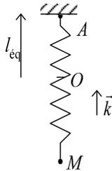
$$z = l_{\text{eq}} - l ; \overline{OA} = l_{\text{eq}} = l_0 + \frac{mg}{k}$$
